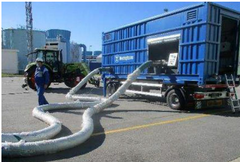
Figure 13: Mobile Spent Fuel Pit Heat Exchanger
