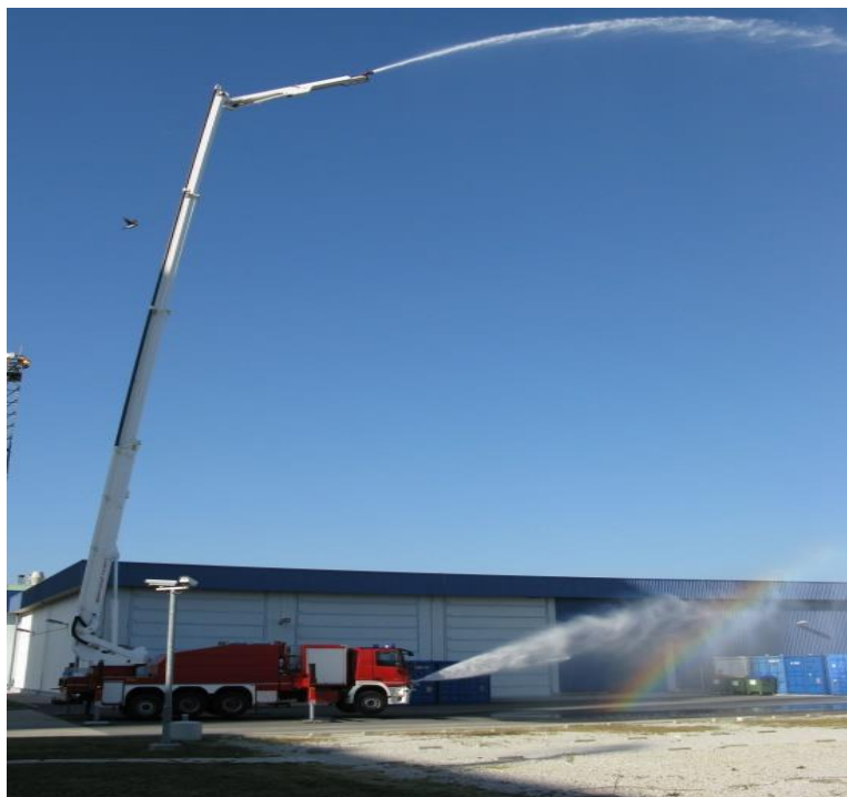
Figure 33: Firefighting Truck with Hydraulic Arm
