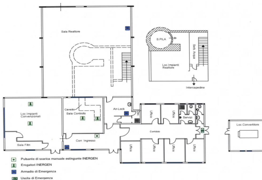
Fig. 3 Automatic Fire suppression system
