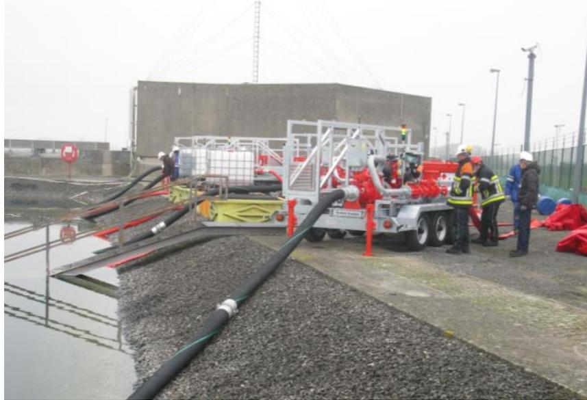
Figure 6 : Mobile pumps training at the Doel NPP in the framework of the CSBO strategy
