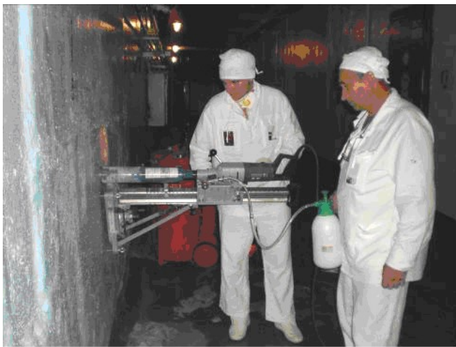
Figure 6.4 Cutting of specimens
