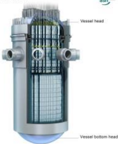
EPR 1650 MW reactor vessel
