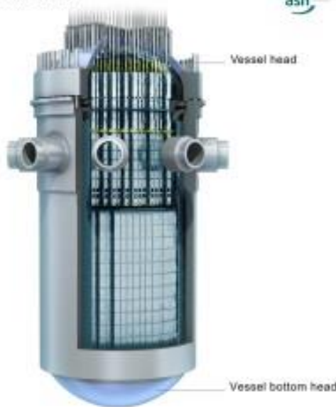
EPR 1650 MW reactor vessel
